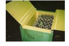
Layer Zerust® Profile Board in between metal parts or objects, or simply set metal parts on top of a Zerust® Profile Board. Next, place metal objects (with the Zerust® Profile Board) inside of an enclosure (such as a Zerust® Bag, or wrap with Zerust® Stretch Film) to restrict airflow.
